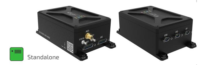
Beta configuration is intended for use as an autopilot for controlling various types of aerial vehicles with all-digital interfaces, as a main navigation system providing data over available digital interfaces or as a supportive navigation system for customer's application which requires positional data.
