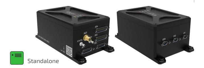
Gamma configuration is intended for use as an autopilot controlling the whole aerial vehicle flight including (but not limited to) engine control, aircraft guidance, mission control, take-off, landing.
